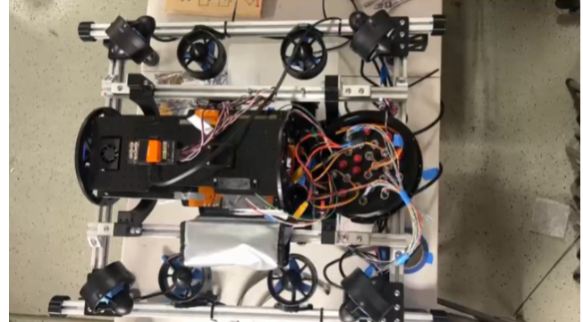
Fig. 6. Unit testing thrusters in final configuration on frame
